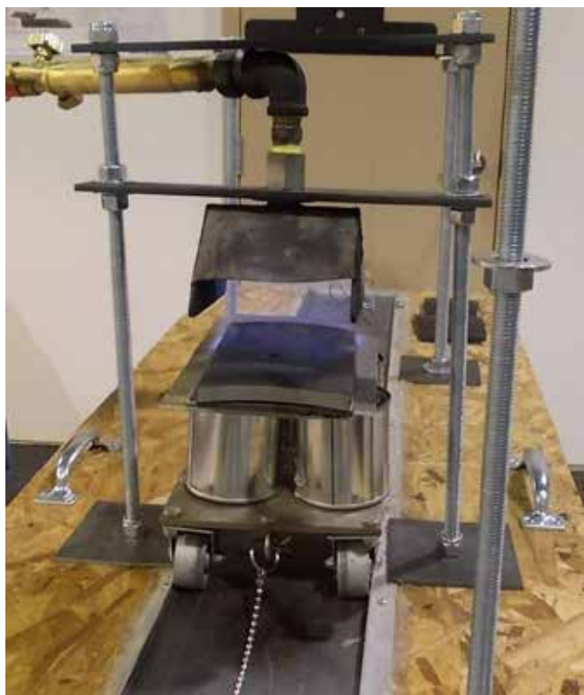
Figure 3. Surface treatment apparatus using Flynn Burner head.
